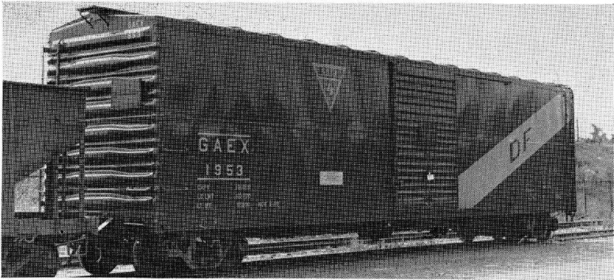
View of the new 50-ton all-steel experimental freight car, 10 of which have been leased by the B. and M. in the hope of safeguarding and expediting valuable freight
