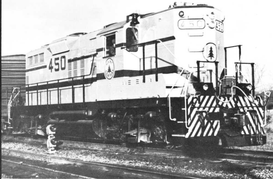
Maine Central No. 450 is the only GP-9 on the roster, and was the last GP-9 manufactured in Canada. The unit was obtained from Algoma Central (No. 171) and because of its weight is limited to yard switching duties at Waterville. Fresh from the MeC shops, the locomotive was photographed by Bill Robertson in Waterville on December 4, 1981.
