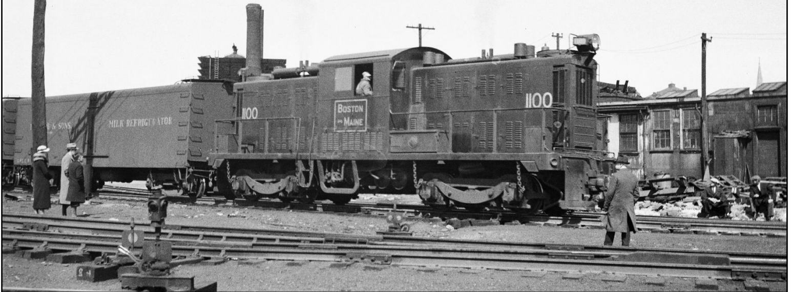
Above: B&M's one-of-a-kind Ingersoll-Rand diesel #1100 works milk cars near Somerville/Charlestown, MA, May 1937. The unique early diesel seems to have attracted quite a bit of attention from a crowd of folks who are likely used to steam power! Robert E. Chaffin photo from the B&MRRHS Archives.
