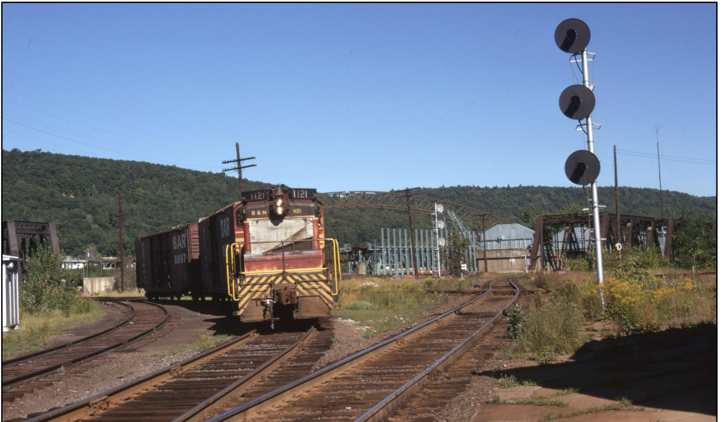
Bellows Falls, VT, Boston & Maine EMD SW1 #1121, the Bellows Falls switcher, is on the connection track between the B&M's Conn River Mainline (foreground) and the Green Mountain Railroad (running left to right in the midground) Notice the diamond crossing where the two lines intersect, between the signals. Benjamin Perry photo.
