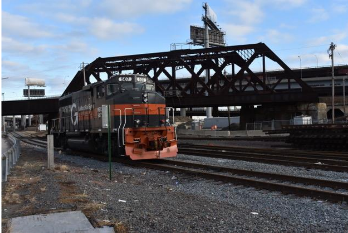
Recently repainted PAR GP40-2W 507 sits outside the Boston Engine Terminal with the old High Line bridge in the background. This bridge carries the B&M New Hampshire main line over the tracks that lead to BET and is soon to be replaced by an upgraded structure. Andrew Riedl photo, 12/26/20.
