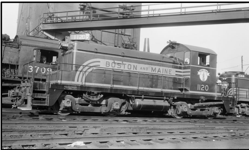
The steam to diesel transition era on the Boston and Maine is well documented in Chaffin's photography. In this October 1953 view at New Boston Terminal, 3-month-old SW1 1120 is assigned to switching duties once likely belonging to now displaced G class 0-6-0 switchers. RS3 1544 and P-3-a class 3709 are awaiting Commuter Rail passenger assignments.
