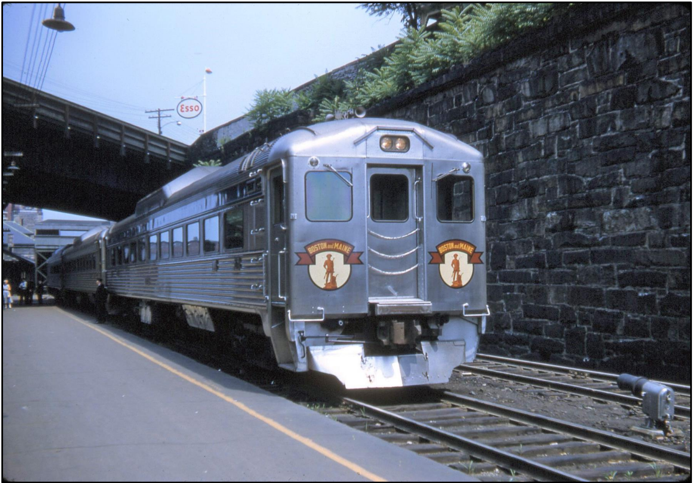
The self-propelled Budd RDC (Rail Diesel Car) made its debut on the B&M on April 27, 1952. The “Buddliners” were immediately successful and soon replaced most locomotive-hauled passenger trains. This photo of an RDC-1 proudly displaying the Minuteman logo was taken at Middlesex Street Station in Lowell by Mason B. Flagg, c.1953.
