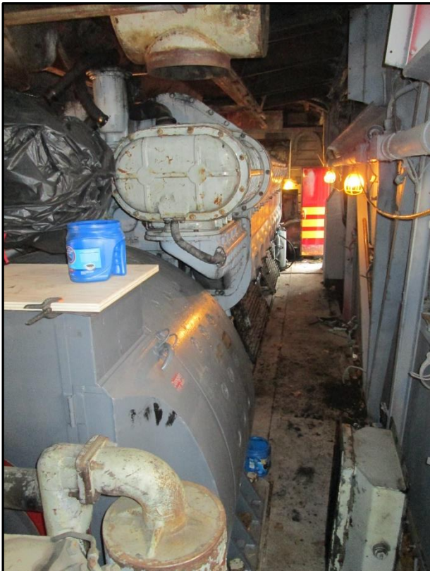
The engine room of 4268 with the recently installed EMD 567 prime mover from donor unit GP9 1757.
