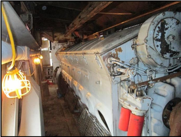
The engine room of 4268 with the recently installed EMD 567 prime mover from donor unit GP9 1757.
