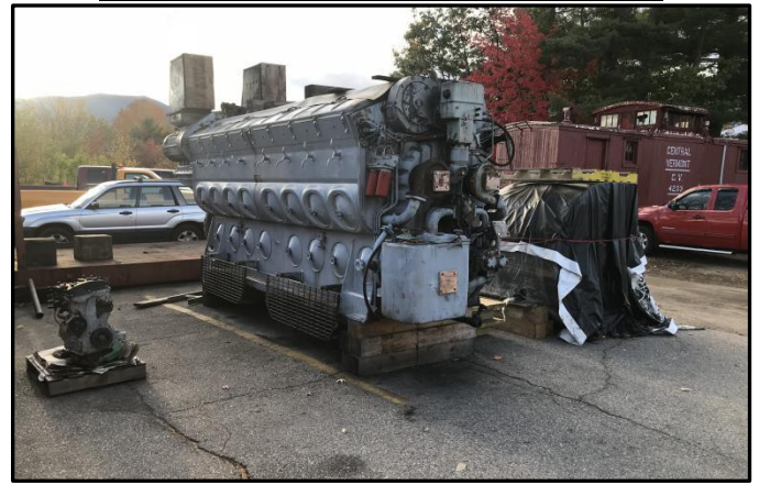
The donor prime mover from CSRX 1757 prior to being installed in 4268.
