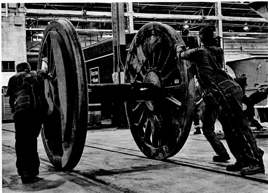
Steamtown volunteers and crew move a set of B&M 3713's drivers. The tender is visible in the background. Photo courtesy of Samantha Kuczynski.
