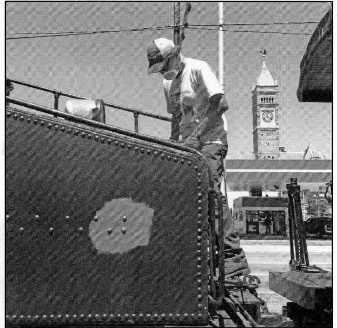
Here is a view of Jim Nigzus removing paint from back of No. 410's tender. Bob Farrenkopf took the picture on June 18, 2016.
