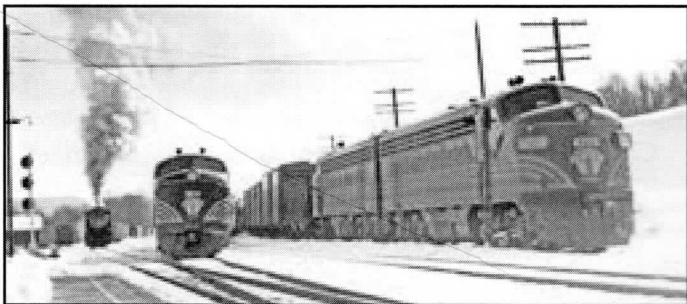
B&M 4268 hauling Symbol Freight SJ-1 with a meet at East Northfield, MA, also featuring B&M E7A #3814 with Train #77, and with CV #467 hauling CV Train #491. The date is March 4, 1950. The photo is by Don Robinson. Note the pilot of B&M #4268 complete with coupler shields as delivered new in October 1949. This was the only B&M EMD F Unit delivered with this passenger style pilot.
