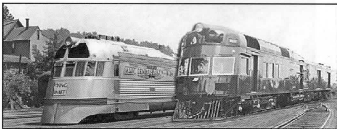
B&M #6000 Flying Yankee diesel-electric Winton engine, 1935
