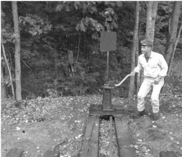
Bruce throwing the switch for siding in the yard.
