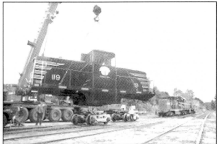
Chris Bertelsen Photo Terry Koller, railroad operations manager at the Coastal Heritage Society's Savannah, Ga. Roundhouse Railroad Museum, left, and Miller Construction crane crew member Mick Stankevich guide Claremont Concord Railroad's General Electric 44 ton locomotive No. 119, suspended from a crane and minus its wheels, onto a flatbed truck at the railroad's shop facilities in Claremont Jct. Restored and freshly painted, the 119, as local train crews call it, and No. 30, an older version of the same locomotive, were sold to the museum after two decades of service in the Claremont Concord
