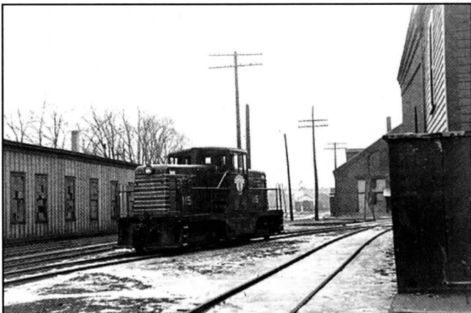
The 44 ton switcher at the Keene roundhouse before starting the day. The engine faced east and the fireman's position was covered by 2 mirrors so the engineer could see the crew.
