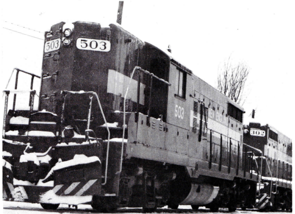
Here's the New England Southern's new power! Ex-Rock Island GP18 and GP7 were at Concord, NH on the first day "fired up" the GP18 503. The GP7 is now in storage pending transfer to the Worcester, MA operation after the first of the year. They are painted green and yellow, the green being close to Burlington Northern green. Photo and story by Harry Frye.
