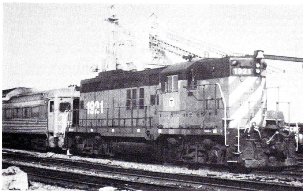
Ex-Burlington Northern GP9 1921 rests between runs at the "interim" North Station. Unit is still in BN green, with only a small "T" decal under the cab window to identify the new owner.
