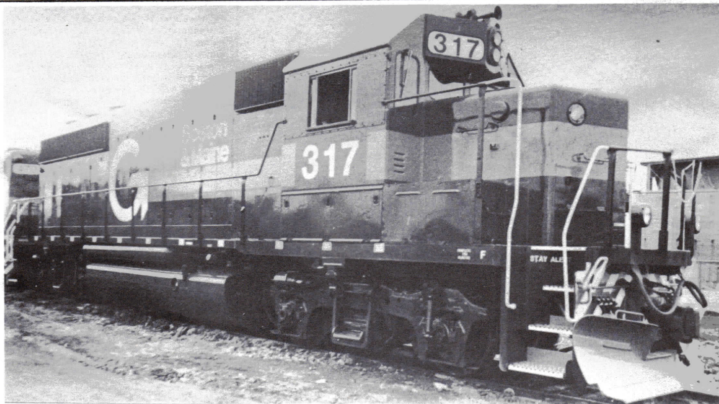
The Boston & Maine Railroad recently unveiled their first Guilford paint scheme. GP40-2 317 carries the colors, and sports new ditch lights and a new Maine Central type Nathan 5 chime horn!!! Photo by Jerry Angier, courtesy of Robertson Books.
