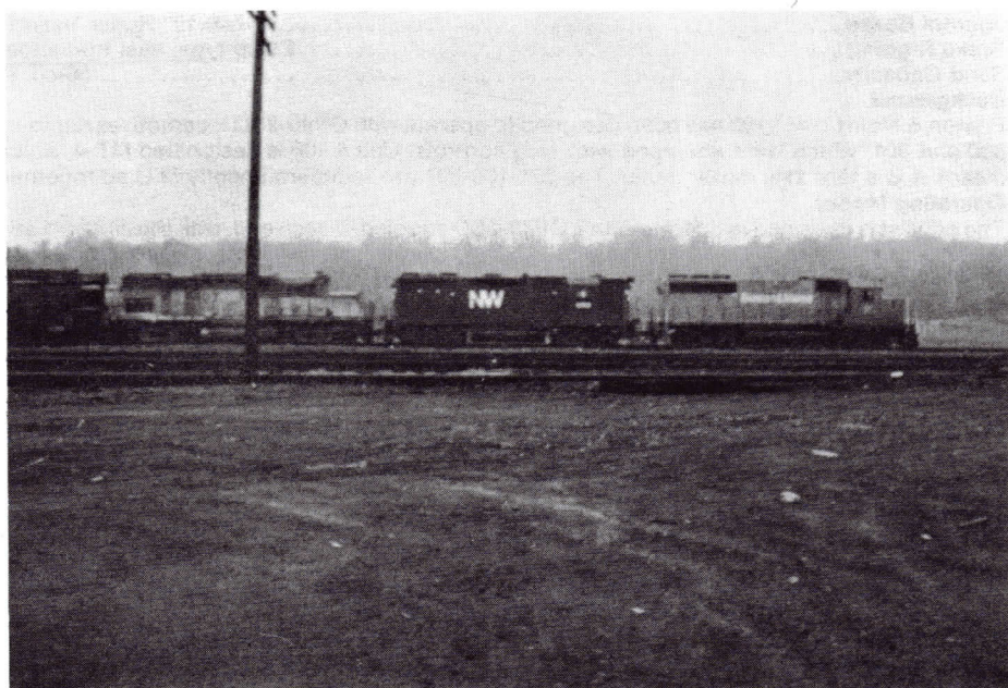
Another typical, boring wash-up leaves East Deerfield yard recently. Power was B&M GP40-2 314, Norfolk & Western GP35 1323 and Delaware & Hudson Alco C-420 407.
