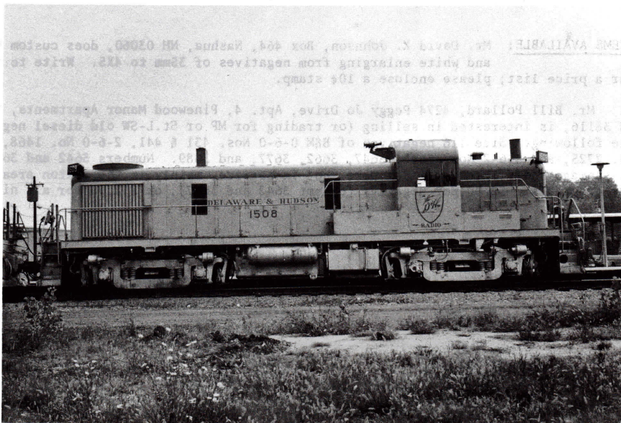
The B&M's steam generator-equipped Alco RS-3 No. 1508 in the lessee's paint scheme, photographed at Rensselaer, New York on Sept. 9, 1974. The D&H is using the unit on the Albany-Montréal portion of the daily Adirondack service. -- Jack Armstrong Adams, Mass.
