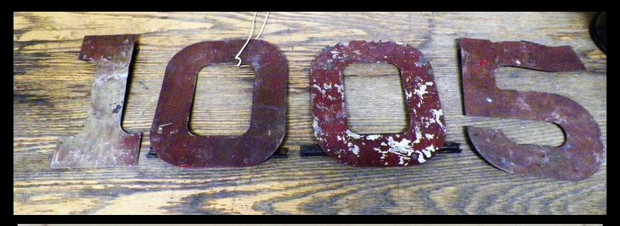
BOSTON & MAINE RAILROAD: Set of train numbers which were mounted on a rod in front of the locomotive headlight to denote the number of the train. (Not the locomotive). Used in the 1885 to 1925 period. Use discontinued in 1925.
