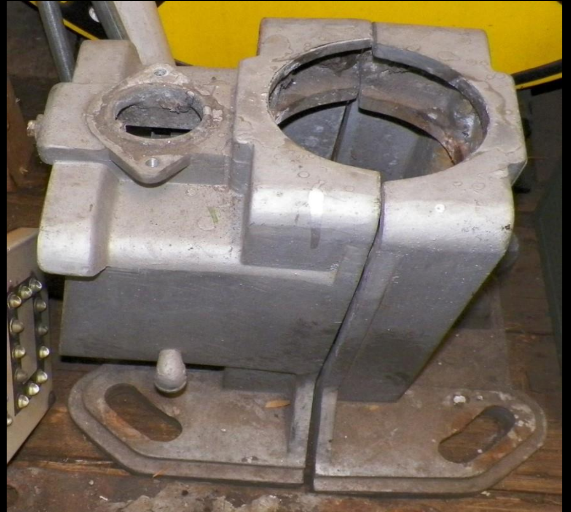
Aluminum Highway Grade Crossing base
