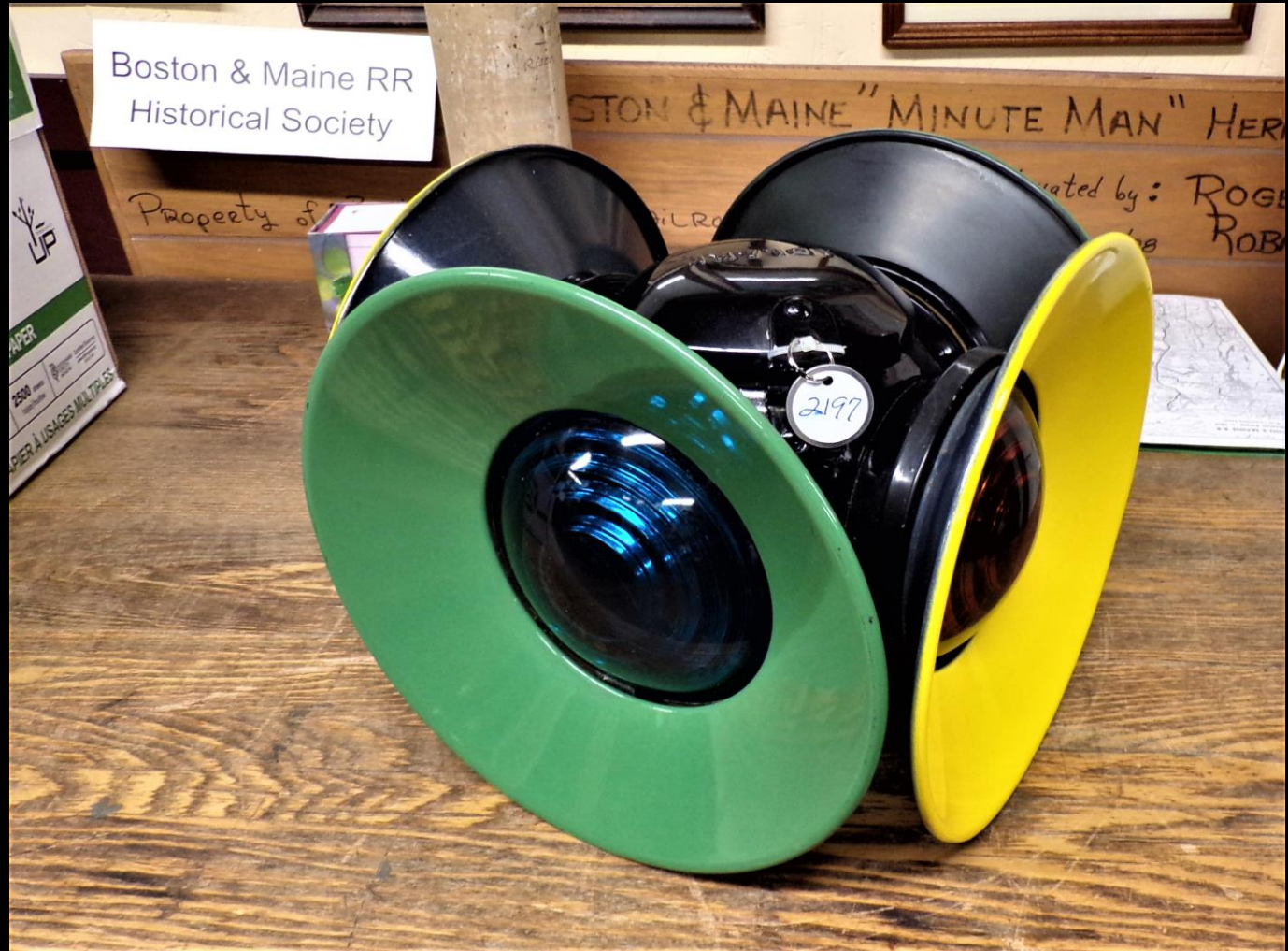
2019 Fixed Globe Lantern w/ Red Globe Adlake Switch Stand Lamp / Green & Blue Lens
