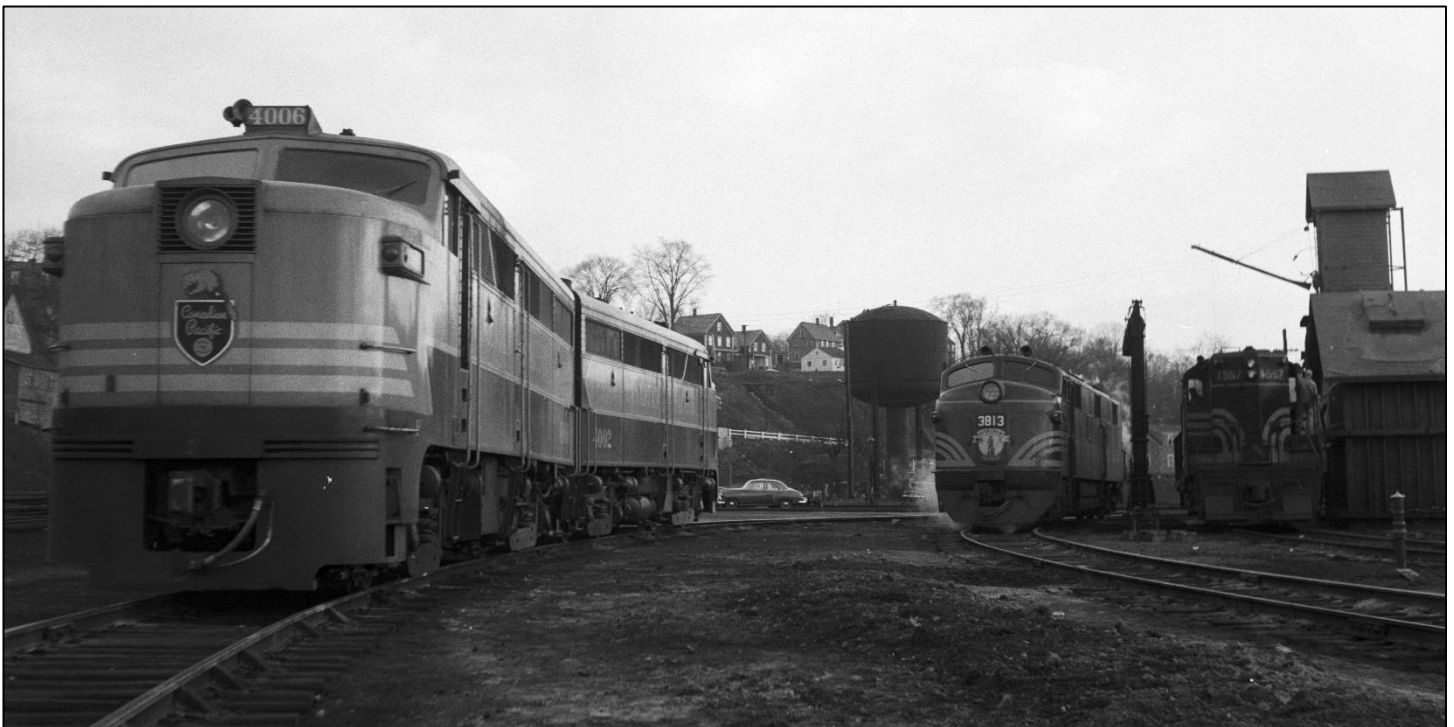
Below: A pair of Canadian Pacific MLW FA-1s rest at the Boston & Maine's Westboro engine terminal in West Lebanon, NH, along with a B&M E7 and a GP7. The Canadian Pacific power was used on their run from Newport, VT to White River Junction. 1950s. Official Boston & Maine Railroad photo, MacMillan/Hutchinson Collection, B&MRRHS Archives.
