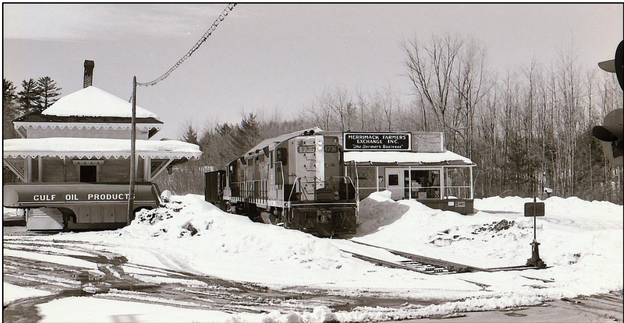
March 9, 1975 – B&M GP9s 1736 and 1747 GP-9's on train ID-2 southbound with a loaded hopper of coal. Apparently, the B&M was unable to deliver the car on the Conway Branch north of Ossipee due to snow conditions. The train symbol DI-1 / ID-2 was a carryover from before October 31, 1972, when the crew had limits to run to Intervale and take rest at North Conway. Now, they turned at either Ossipee or Mount Whittier and returned to Dover. Bruce S. Nelson photo, courtesy.
