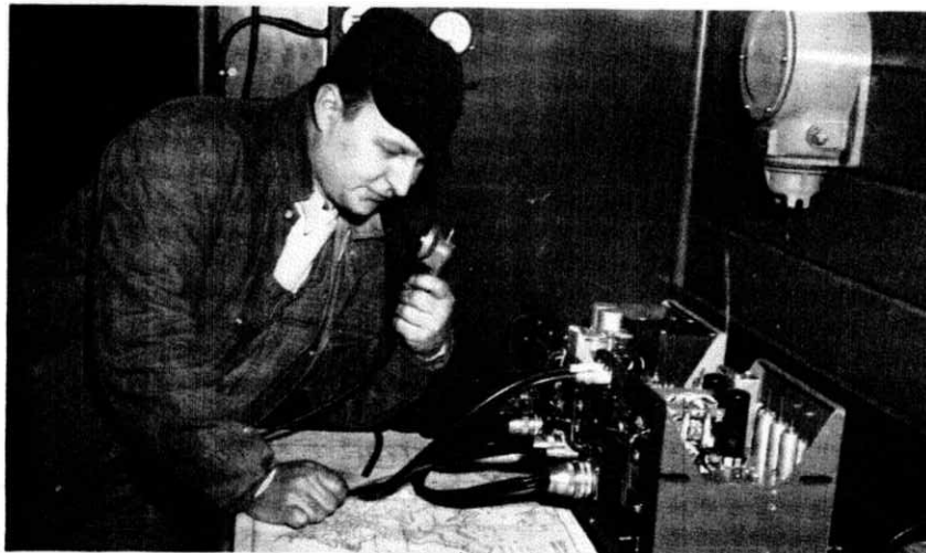
Caboose talking with head end by radio phone on a Boston and Maine freight train
